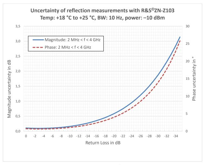
Uncertainty of reflection measurement with R&S®ZN-Z103 calibration unit.
