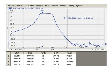
The VNA has a large frequency range with the option of frequency scan segmentation. This allows optimal use of the device, for example, to realize the maximum dynamic range while maintaining high measurement speed.
