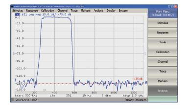
Typical dynamic range of 135 dB is achieved through the entire frequency range (at 10 Hz IF bandwidth). Seen here is the maximum dynamic range achieved when using IFBW 10 Hz and an output power level of 3 dBm.
