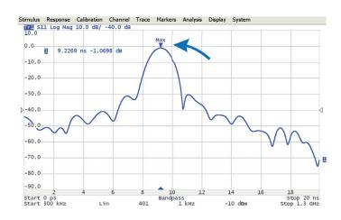
Here, built-in time domain analysis allows the user to detect a physical impairment in the antenna feeder.
