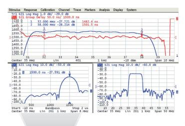
Time domain analysis allows measurement of parameters of SAW filters such as the signal time delay, feedthrough signal suppression.
