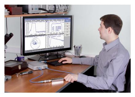
The Planar TR1300/1 VNA is an S-parameter vector network analyzer designed for operation with an external PC. It connects to any Windows-based computer via USB and delivers accurate testing and measurement through a platform that can keep up with constant advancements as well as be remotely accessed.
