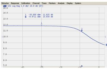
The power sweep feature turns compression point recognition, one of the most fundamental and complex amplifier measurements, into a simple and accurate operation.
