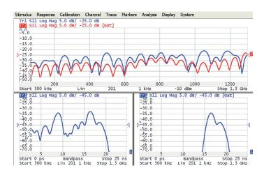
This function mathematically removes unwanted responses in the time domain, which allows the user to obtain frequency response without influence from fixture elements.
