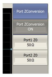
This function converts the S-parameters measured at the 50  $\Omega$  port into values, which could be determined if measured at a test port with arbitrary impedance.
