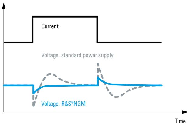
Power supplies usually respond to abrupt load changes with overshoot and slow recovery times. Thanks to specially optimized control circuits, the R&S®NGM200 series achieves recovery times of  $< 30 \mu\text{s}$ .
